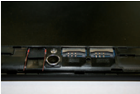
Proper microSD card installation
